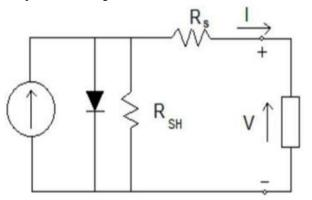
Fig. 1: Mathematical model of PV module
